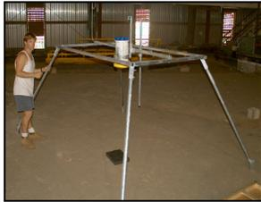
The Wave Boundary Layer Profiler (WBLP) instrument platform prior to lab testing at J.K.K Look Laboratory.
